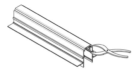
3. Drill the power cable entry holes and remove the chamfers.
