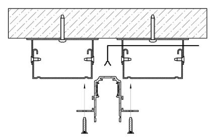
8. Install the plasterboard close to the track walls and secure it with screws. Bond a layer of fiberglass mesh. Cover the plasterboard with putty to make level with the track walls.
