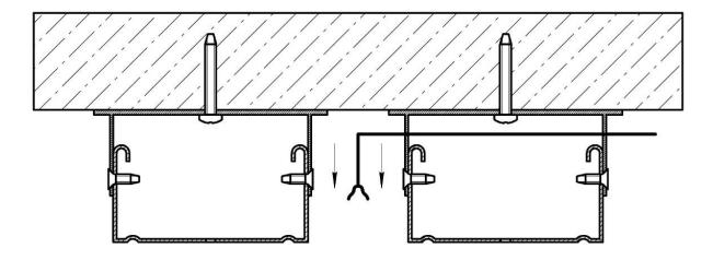
7. Install the track into the mounting slot and secure it with screws.
